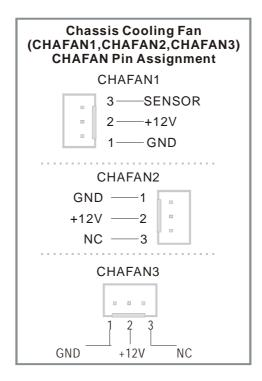
*Note:* CPU cooling fan must be installed to prevent the CPU from overheating and ensure system stability. Chassis cooling fan is optional, depending on whether there is cooling fan in your chassis.
